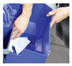
2.8 If needed, pull black tray forward at bottom of machine and wipe clean. Then, push tray forward and return waste bucket to machine.
