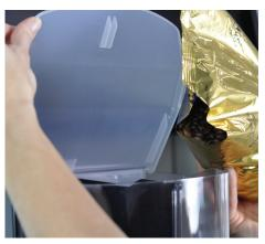
2.6 Remove drip tray assembly from bottom of machine. Then, remove drip platform and clean drip tray with mild soap and warm water. Dry thoroughly, reinstall drip platform, and set aside.
